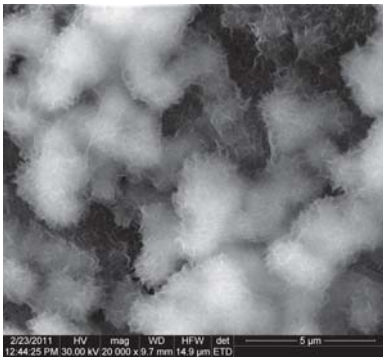
Fig. 5. SEM microphotograph showing the apatite deposits onto the surface of SF/PAAm/MWCNT-COOH hydrogels (SF/PAAm 10/90, v/v), incubated in SBF 1x
