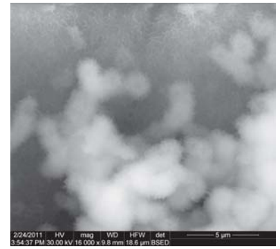
Fig. 7. SEM microphotograph showing the apatite deposits onto the surface of SF/PAAm/MWCNT-COOH hydrogels (SF/PAAm 50/50, v/v), incubated in SBF 1x
