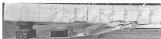
(c) Shear span-depth ratio of 2.57 (Specimen 1L0-1000)
