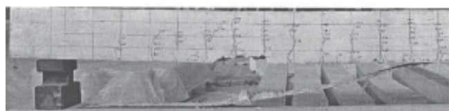
(b) Shear span-depth ratio of 3.71 (Specimen 1L0-600)
