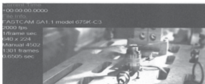
Fig. 3. Measurement of rotation speed using high speed video camera
