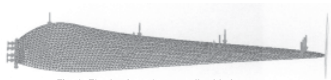
Fig. 8. The load on the propeller blade
