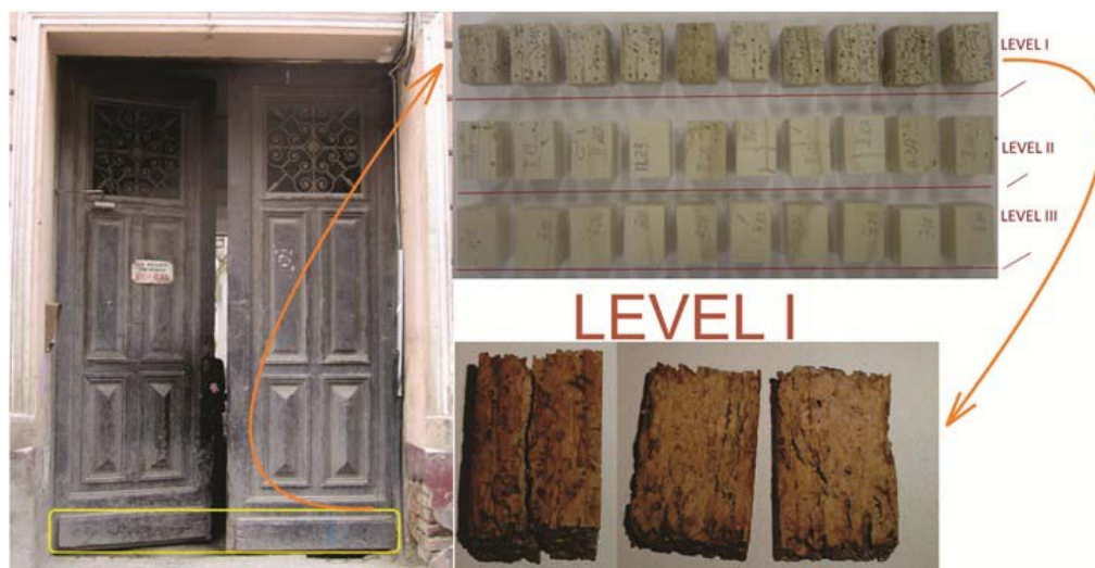
Fig.1. The gateway before restoration: bottom wooden elements used as experimental material; division according to initial conservation levels
