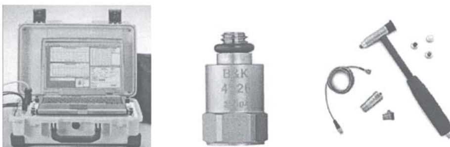
Fig. 7 The experimental set-up: a. Pulse system; b. Piezoelectric accelerometer; c. Modal hammer
