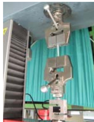
Fig. 3. Zwick Roell Stand 005 for tensile test compression 5 kN
