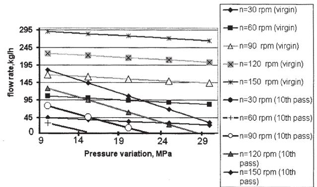
Fig. 1. Flow rate versus pressure variation for PP at 200°C (virgin, 10th pass), model with leaks over the flight tip ( $\delta_s = 0.6$ mm, in the case  $\frac{\partial p}{\partial z} > 0$ )
