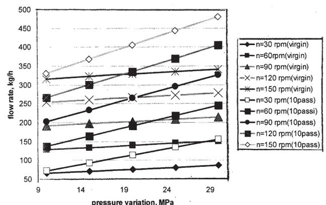
Fig. 2. Flow rate versus pressure variation for PP at 200°C (virgin, 10th pass), model with leaks over the flight tip ( $\delta_s = 0.6$ mm), in the case  $\frac{\partial p}{\partial z} < 0$
