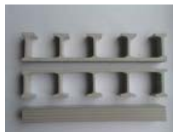
Fig. 1. Glass fibers-reinforced isophthalic polyester resin pultruded T-profiles
