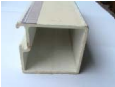
Fig. 2. Glass fibers-reinforced isophthalic polyester resin pultruded hollow square profile
