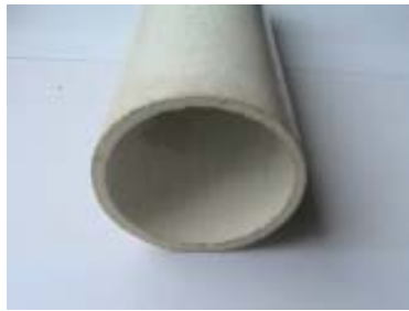
Fig. 3. Glass fibers-reinforced isophthalic polyester resin pultruded hollow tubular profile
