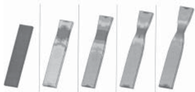
Fig. 5. Numerical simulation of specimen's traction test
