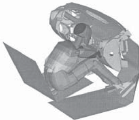
Fig.8. Passengers impact with the cockpit module
