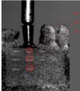
Fig. 3. Key points considered: P2 - in the implant neck area, P5 - at about 1/3 of the implant, P8 - in apical area of the implant
