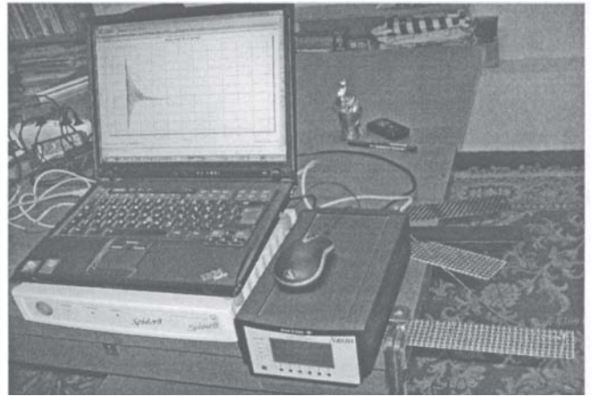
Fig. 4 Experimental set-up for determination of damped free vibrations
