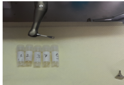
Fig. 3. The reciprocating system with Periotor insert, together with the instrumented samples
