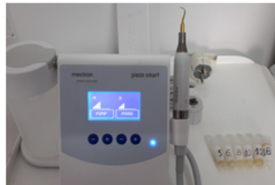
Fig. 2. The ultrasonic piezoelectric system, together with the instrumented samples
