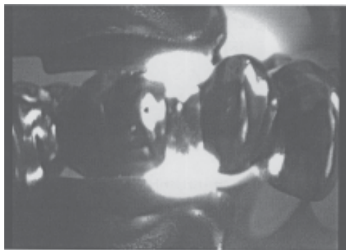
Fig. 6. Transillumination investigation of the interface between the polymer and metal components of the fixed partial sample number 11: no defect is detected inside the polymeric material because of the wrong positioning of the fixed partial prosthesis related to the Diagnocam system..
