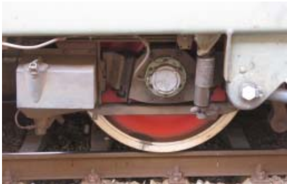
Fig. 2. Primary suspension of the electrical locomotives manufactured in Romania
