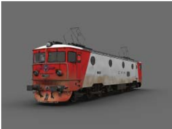
Fig. 1. Six axes Romanian electrical locomotive
