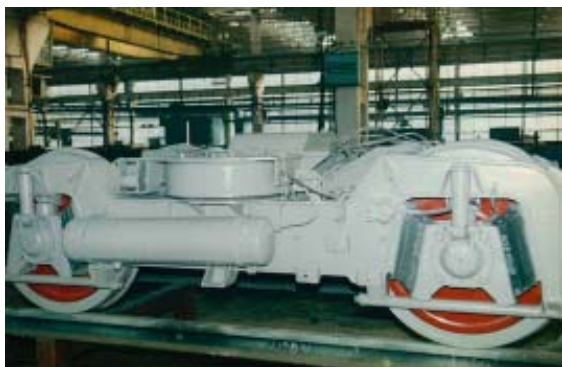
Fig. 3. Primary suspension of the metro trains manufactured in Romania
