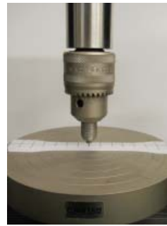
Fig. 3. Geometry of the injection molding specimen (a) and cylindrical indentation set-up (b)
