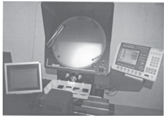
Fig. 9. Warpage measurement with optical machine equipment
