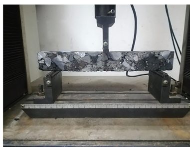
Figure 3. Bending failure test
