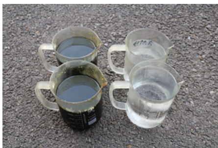
Figure 1. Isocyanates (black material) and polyether polyols (white material)
