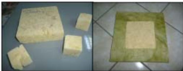
Fig.6. Sample of polyurethane foam (a) and test piece for determination of thermal conductivity (b)
