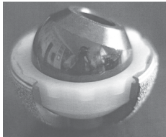
Fig. 3. Zirconia / polyethylene friction couple (metallic femoral head with a zirconia layer in an acetabular cup – the metal back was cut-off in order to visualize the polyethylene cup inside it)
