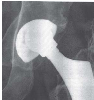
Fig. 2. Worn polyethylene acetabular cup – antero-posterior X-ray view of a cemented total hip prosthesis
