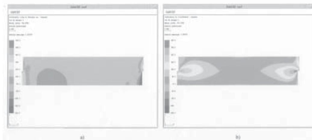
Fig. 3. Stress distribution in cylindrical bonded joint modeled with quadrangles elements for  $f = 100$  MPa:
