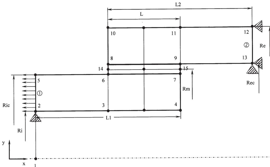
Fig.1. CAD diagram of a cylindrical adhesive bonded joint
