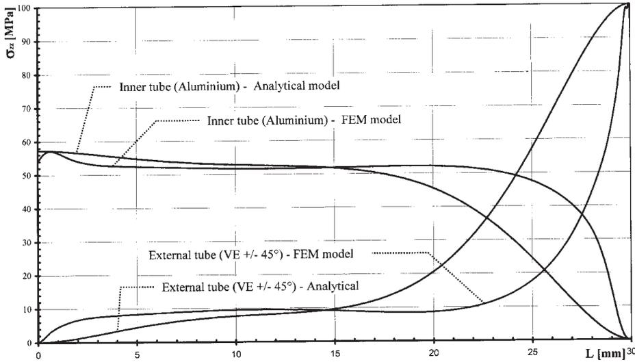
Fig. 4. Load transfer in an AU 2024 T3-AV 119-VE ±45° assembly
