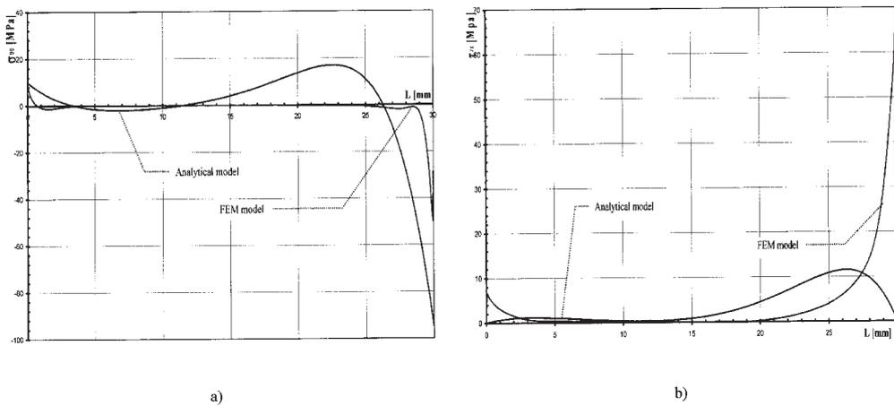
Fig. 5. Stress distributions in the adhesive layer of a cylindrical assembly AU 2024 T3-AV 119-VE ±45° for  $f = 100$  MPa: a) The orthoradial stress ( $\sigma_{\theta\theta}$ ); b) The shear stress ( $\tau_{rz}$ ).
