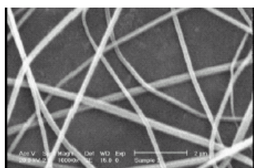
Fig.4.SEM micrograph and fiber distribution of 12wt% of silk at 15 KV and 25° C
