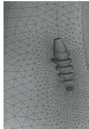
Fig. 4. The overall aspect of model A meshing (left); a detail of the exit area of the lateral column screw (right)
