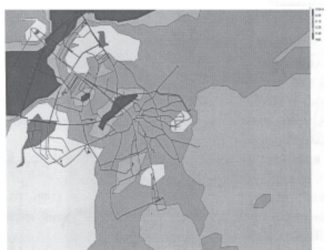
Fig. 10.b. The percentage of residual chlorine in the distribution network - Scenario 2 (consumption 75%)
