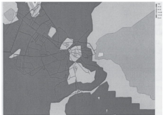
Fig. 11c. The weight for age water distribution network pipes - Scenario 3 (50% consumption)
