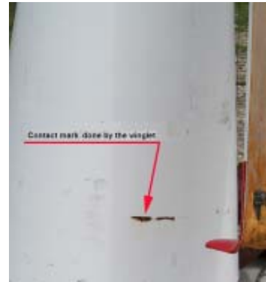
Fig. 2. Pictures of wind turbine after the incident a) lateral view; b) front view ; c) zoom on the impact zone
