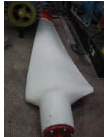
Fig. 3 The least damaged blade on the shell, but having the shaft broken
