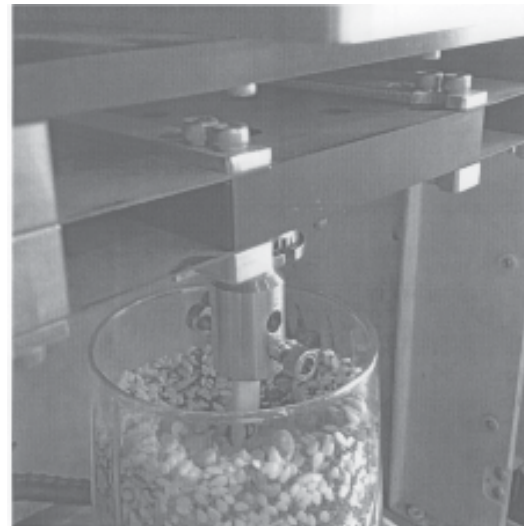
Fig. 3. Bite simulation on a dry mixture of poppy, sesame and sunflower seeds
