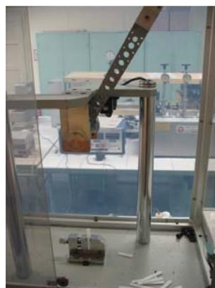
Fig. 5 Izod impact tester, Model PENDOLO P400, HAMMEL/England
