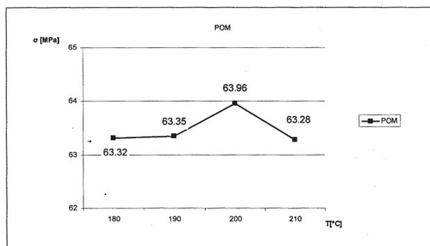
Fig. 10 The tensile strength at break variation ( $\sigma$ ) depending on the processing temperature for POM
