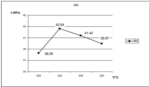
Fig. 8 The tensile strength at break variation ( $\sigma$ ) depending on the processing temperature for ABS
