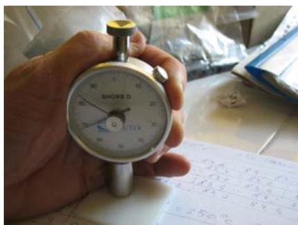
Fig.2 Shore Type D Durometer, Model SAUTER HB/Germany
