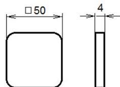
Fig. 3 Specimen model for hardness tests
