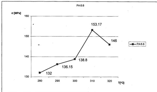
Fig. 9 The tensile strength at break variation ( $\sigma$ ) depending on the processing temperature for PA 6.6
