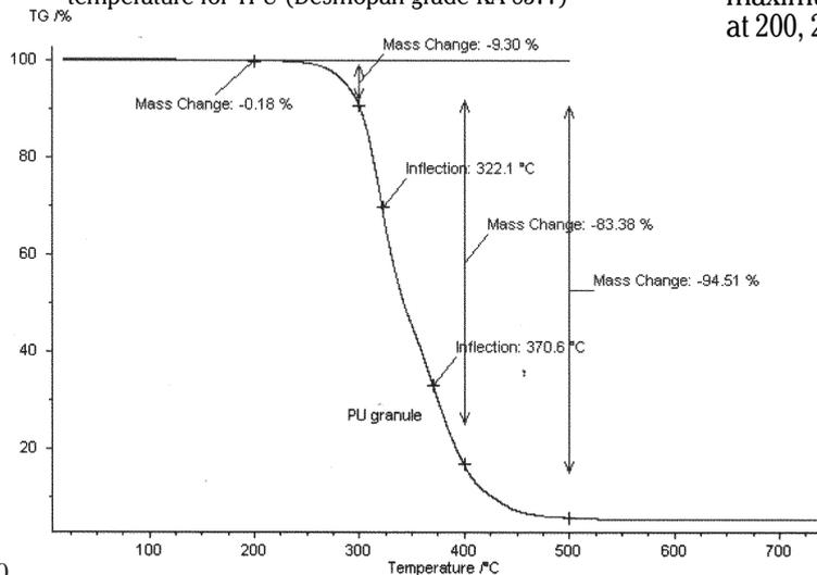
Fig.4. TG diagram for TPU grains
