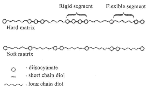
Fig.1 Structure of thermoplastic polyurethane (TPU) [2]
