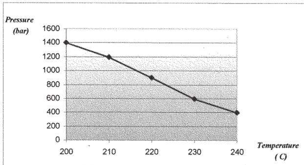
Fig.2. Dependence of in-mould pressure peak on the real injection temperature for TPU (Desmopan grade KA 8377)
