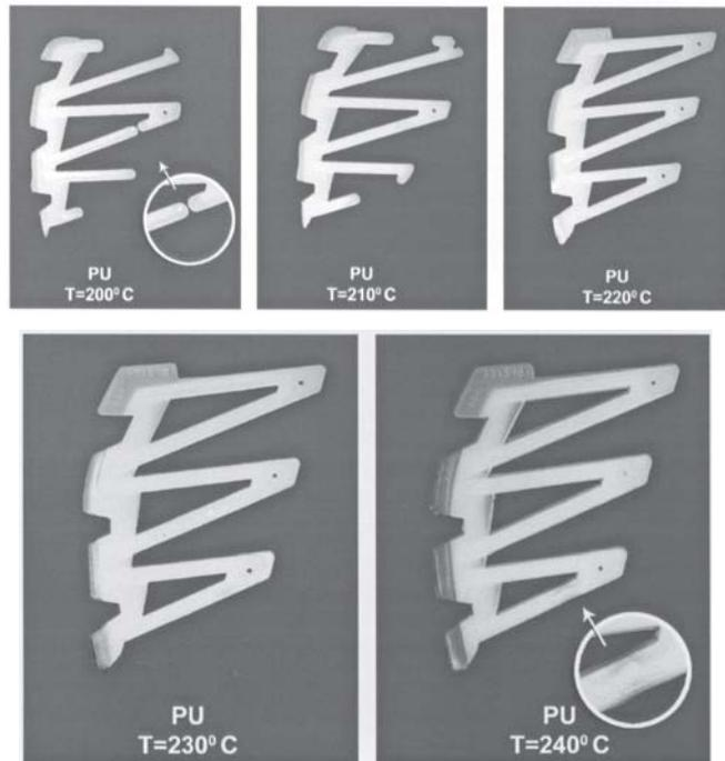
Fig.3. Influence of injection temperature on the quality of TPU moulded parts (grade Desmopan KA 8377)
