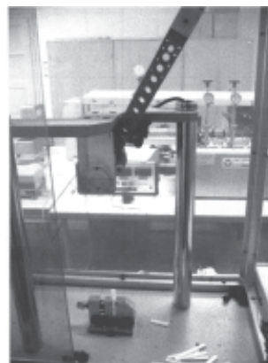
Fig. 6. Device for determining Izod shock properties, PENDOLO P400 model, HAMMEL/ England
