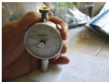
Fig.3. Shore D durometer, model SAUTER HB/ Germany
