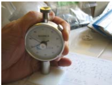
Fig.2. Shore Type D Durometer, Model SAUTER HB/Germany
