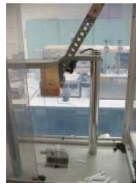
Fig.5. Izod impact tester, Model PENDOLO P400, HAMMEL/England
