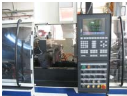
Fig.1. ENGEL CC 100 Type ES 80/50 HL injection machine
