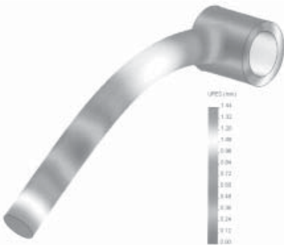
Fig. 7. Displacements distribution on the optimized rod
