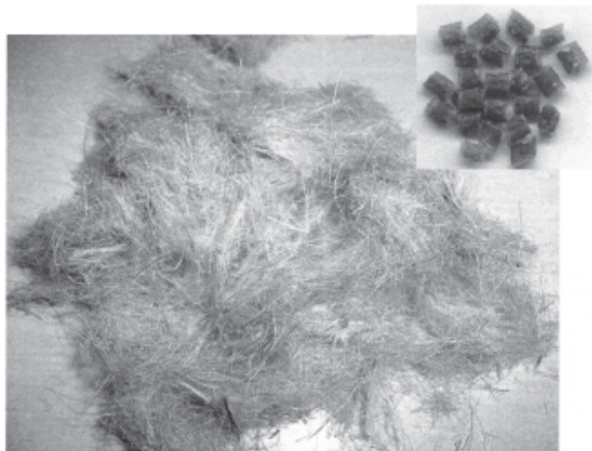
Fig. 1. Short cut AS treated hemp fibers (AS-HF); inset - Granules of PP with AS-HF obtained on the twin screw extruder
