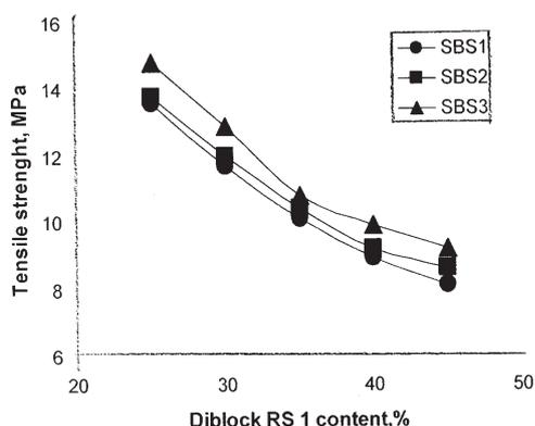
Fig. 4. Tensile strength dependence on SBS molecular weight and RS 1 content.
