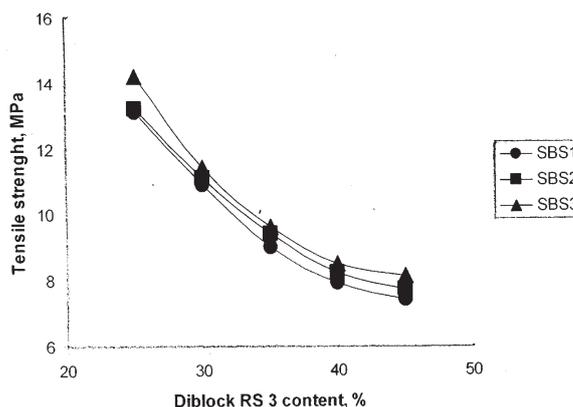
Fig. 6. Tensile strength dependence on SBS molecular weight and RS 3 content
