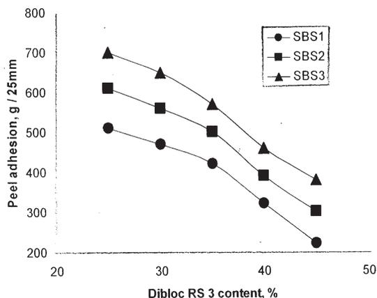
Fig. 12. Peel adhesion dependence on SBS molecular weight and RS 3 content
