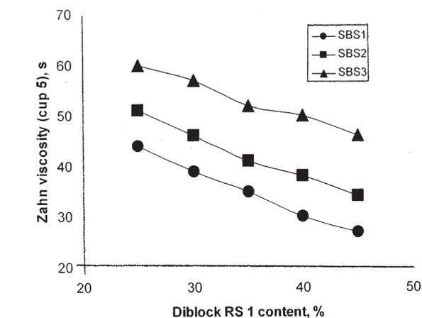
Fig. 1. Dependence of masking solution viscosity on SBS molecular weight and RS 1 content
