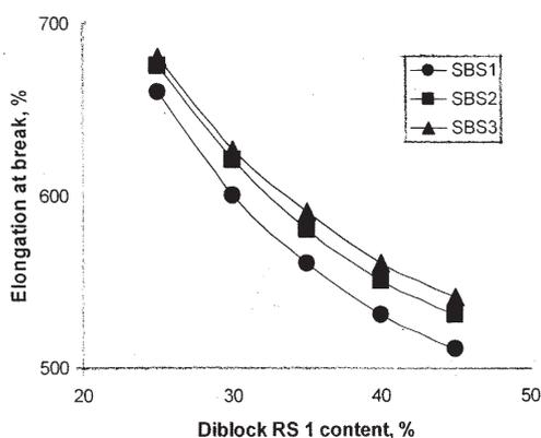
Fig. 7. Elongation at break dependence on SBS molecular weight and RS 1 content.
