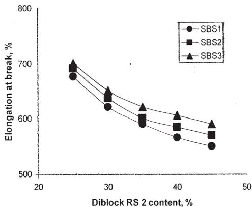
Fig. 8. Elongation at break dependence on SBS molecular weight and RS 2 content.
