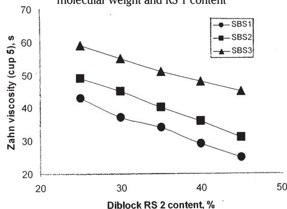
Fig. 2. Dependence of masking solution viscosity on SBS molecular weight and RS 2 content.
