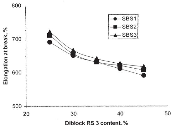
Fig. 9. Elongation at break dependence on SBS molecular weight and RS 3 content
