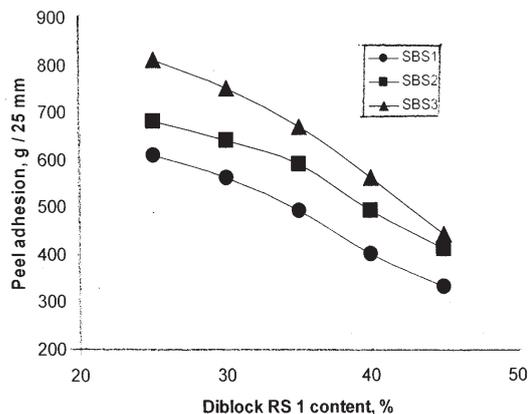
Fig. 10. Peel adhesion dependence on SBS molecular weight and RS 1 content
