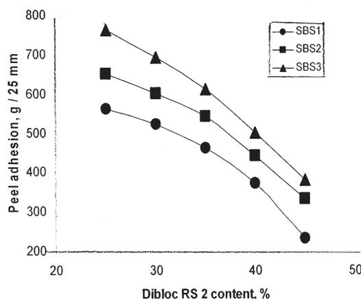
Fig. 11. Peel adhesion dependence on SBS molecular weight and RS 2 content
