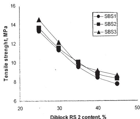
Fig. 5. Tensile strength dependence on SBS molecular weight and RS 2 content.
