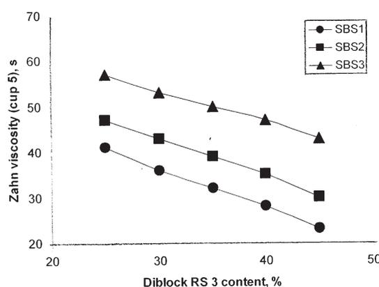
Fig. 3. Dependence of masking solution viscosity on SBS molecular weight and RS 3 content
