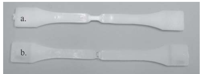
Fig. 2. Tested mono-component specimens: (a) HDPE ( T_{melt} 255°C, T_{mold} 50°C), (b) LDPE ( T_{melt} 255°C, T_{mold} 50°C)
