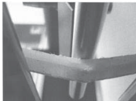
Fig.3. Al 2 O 3 (5% volume fraction) particle reinforced multi phase composite sample after a 3-point bending test (closer view)
