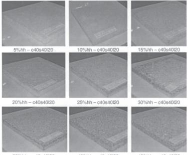
35%hh - c40s40l20 40%hh - c40s40l20 45%hh - c40s40l20 where hh=hemp hurds, c = cement, s = sand, l = lime; and the figures are percentages from the total mass of mineral binder
