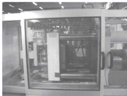
Fig.1. Injection machine KRAUSS MAFFEI KM65-160C1
