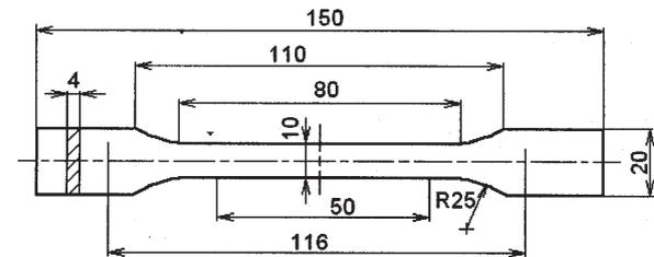
Fig. 7 Specimen model for tensile strength at break testing
