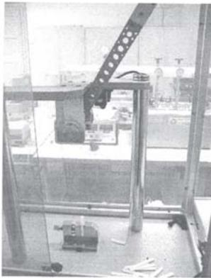
Fig. 5 Izod impact tester, Model PENDOLO P400, HAMMEL/England
