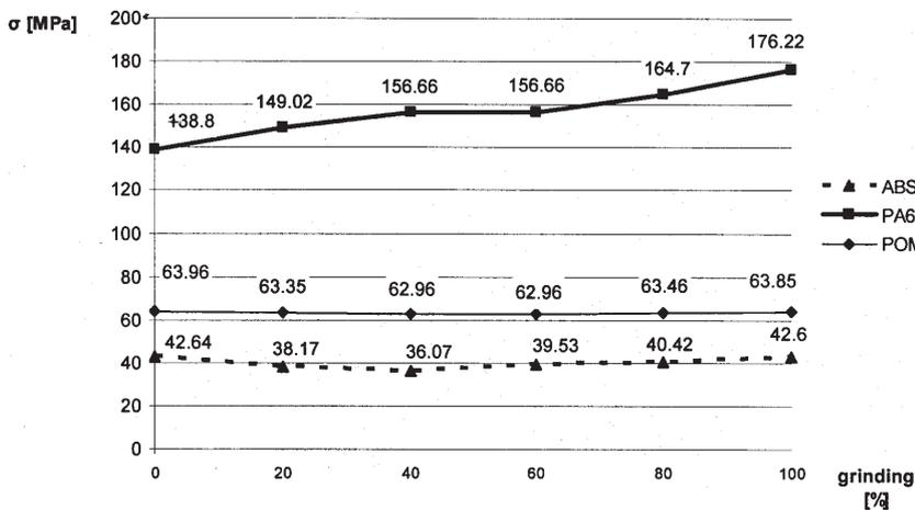
Fig. 8 The tensile strength at break variation ( $\sigma$ ) depending on the grind percentage in the tested samples of ABS, PA 6.6 and POM
