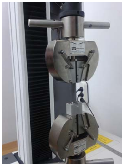
Fig. 1. Instron Universal Testing Machine type 3366, 10 kN
