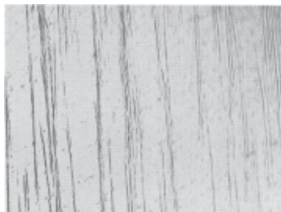
Fig. 17. Metallographic microscopic image of the FGP surface
