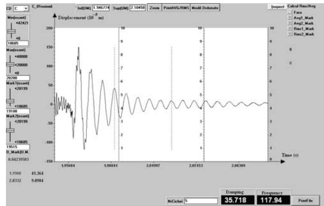
Fig. 5. Experimental recording of damped vibration for a bar with 40 mm width, with core made of polypropylene honeycomb and exterior layers made of epoxy resin reinforced with: fiber-glass fabric a); carbon-fiber fabric b)
