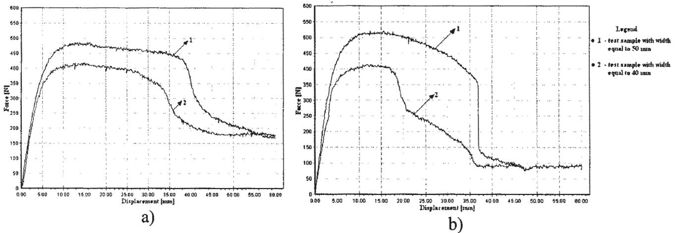
Fig. 3. The dependence between the force applied by the indenter roller and the displacement at the middle of the sample, for samples with core from polypropylene honeycomb, the reinforcement of the exterior layers being made with: a) fiber-glass fabric; b) carbon-fiber fabric
