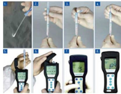
Fig. 1. Working steps using SURE II for ATP assessment
