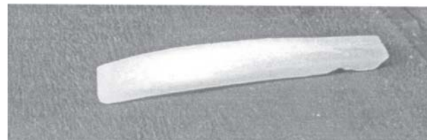
Fig. 7. Akriat-R sample treated at 650 W and 5 min. It can be seen that the surface texture is coarser and the sample is bent
