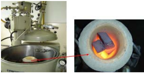
Fig. 6. Balzers furnace used for Cu-Zn alloys elaboration.
