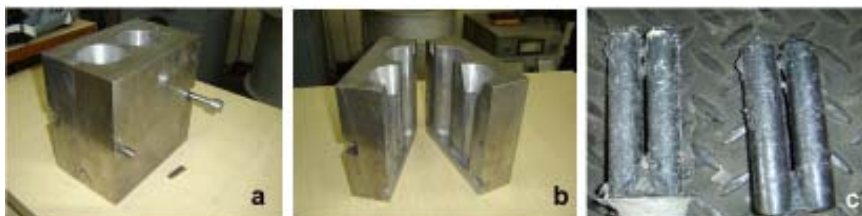
Fig. 5. Casting mold – assembled (a) and disassembled (b) and respectively the elements extracte from the mold casting (c)
