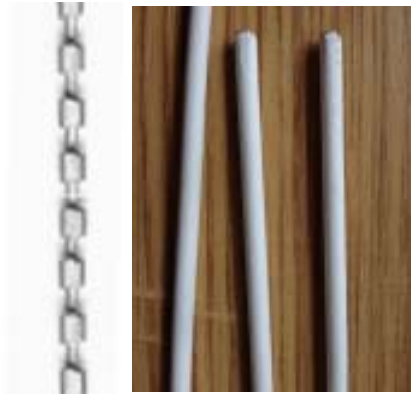
Fig. 9. Experimental electrode extracted from mold, with partial flux deposition and respectively the final welding-brazing electrode
