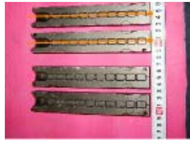
Fig. 8. General aspect of semi-molds, used for flux coating deposition on electrode wires.
