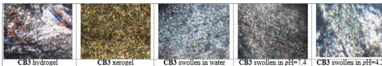
Figure 6. POM microphotographs of CB3 hydrogel and xerogel swollen in media of various pH for 3 h, acquired at room temperature (200x magnitude)
