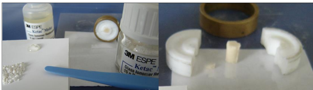
Figure 3. Preparation of specimens for testing
