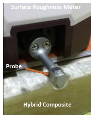
Figure 3. Measurement of surface roughness
