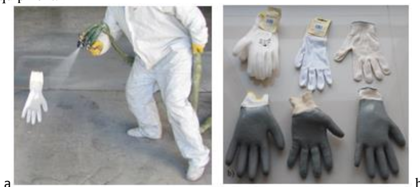
Fig. 1. a) Pulverization of PUC on support layers; b) Protection gloves before and after treatment
